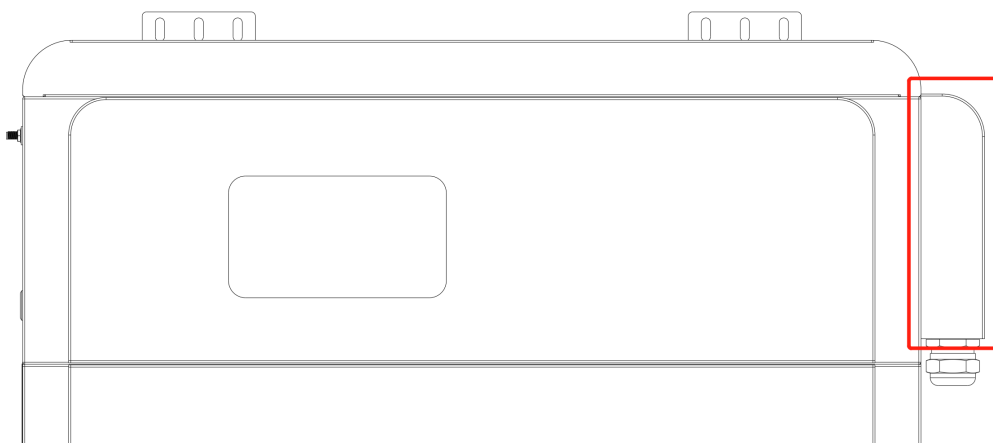
Figure 3.6.1. Removal position of the battery control module
