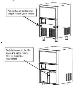
⚠ Note: Be careful when doing the condenser cleaning as the edges of the fins are sharp.
